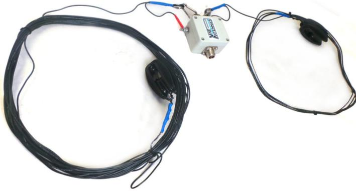
A traditional Dipole is a half-wavelength radiator, fed in the Centre with two equal length legs, the Off-Centre-Fed Dipole is a Dipole whose feedpoint is at a point removed from the centre of the antenna. A traditional dipole is fed in the centre with 50-ohm coax, or more correctly through a 1:1 balun, whereas the off-centre fed dipole is fed through a 4:1 balun. **Specification]** Bands:
